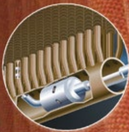
OD Scanning for Tube Wall Thickness
